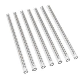
ECS splice protector sleeve is specifically made to accommodate the bare fibers and provide mechanical and environmental protection for fusion splices. Optimal design for simple and correct fiber entrance with hot melt adhesive especially developed for optimal flow. Transparent heat shrinkable tube for simple installation verification and short installation cycle and compatible with most common ovens
