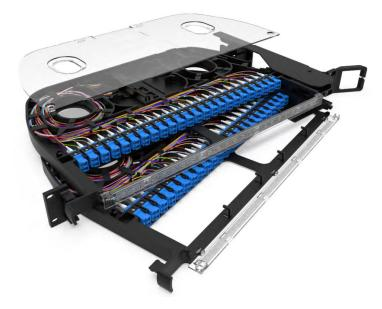
Pivot Patch Panel is an innovative and high density design to accept 24 SC Simplex/LC Duplex adapters in each of two ½ RU trays within 1U space (**Up to 96FO in LC**). Each tray effectively manages the incoming fibers, pigtails and splices. Each tray offers individual pivoting up to 120° to ensure easy access during installation or rework without any interference with the existing cable or fibers.
