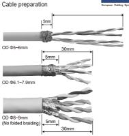
Insert cable through cable gland, follow the Cable Preparation according to cable used. Fan out all four pairs and cut the conductors as shown.
