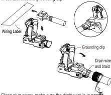
Close plug cover, make sure the drain wire is in proper contact with grounding clip on plug. Screw on the cable gland to fasten and complete installation.
