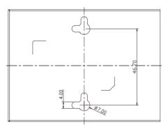
**Step 3:** Hang the LRE-101 on the screws from the wall.
