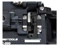
Position the fiber so that it is past the Cleaving Blade. Then, close the Fiber Clamp and Cover Plate to hold the fiber in place. Ensure the fiber is straight and even before cleaving. 3. Gently push the Sliding Block to the back of the unit only once to cleave the fiber.
