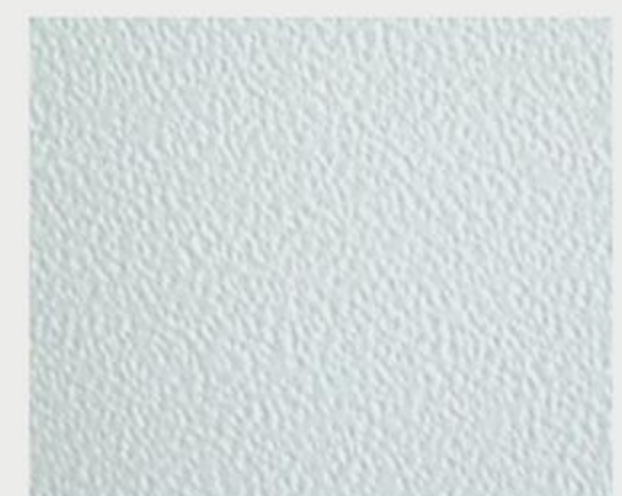
Powdered surface with textured stove enamel
