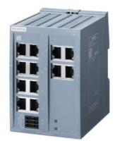
SCALANCE XB112 unmanaged IE switch, 12x 10/100 Mbit/s RJ45 ports, for setting up small star and line topologies; LED diagnostics, IP20, Redundant power supply, 24 V AC/DC Manual available as a download
