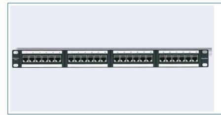
The Deca <sup>10</sup> RapidNet panel accommodates four 6-way Deca <sup>10</sup> cassettes, allowing 24 Cat6A connections per 1U of space. The integral earthing plate grounds each cassette helping to guarantee 10G performance by giving continuity of the 360° shielding.
