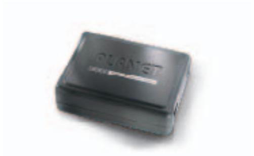
For cost-saving and well power management, PLANET releases a new Power over Ethernet splitter - POE-151S. The POE-151S is an IEEE 802.3af Power over Ethernet device that split the 48V DC over the Ethernet cable into 5/9/12V DC power output. Working with the IEEE 802.3af power source equipment (PSE), the POE-151S frees the device deployment from restrictions due to power outlet locations, which eliminate the costs for additional AC wiring and reduces the installation time.
