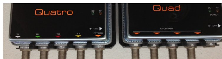
F-connectors with polarities + TER (QUATRO) / universal outputs (QUAD)
