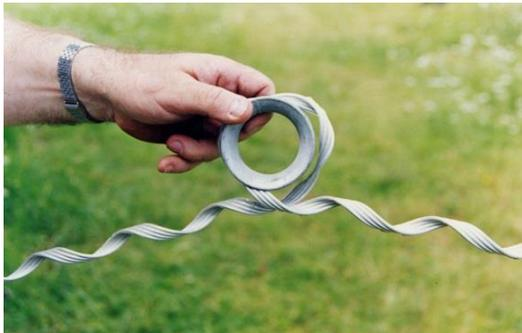
2. Insert the round thimble into the loop of the tangent support.
