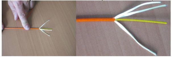
Step 3: Thoroughly shave off one of the deformations by using the knife as shown.
