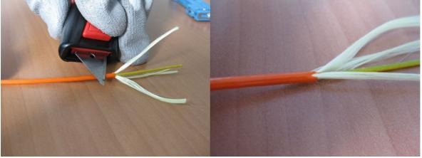
Step 4: Use the tensile strength element at the point you shaved off the deformation as a ripcord to open the Low Friction Jacket the required length. During this process keep the fibre unit and the other tensile strength elements tightly.
