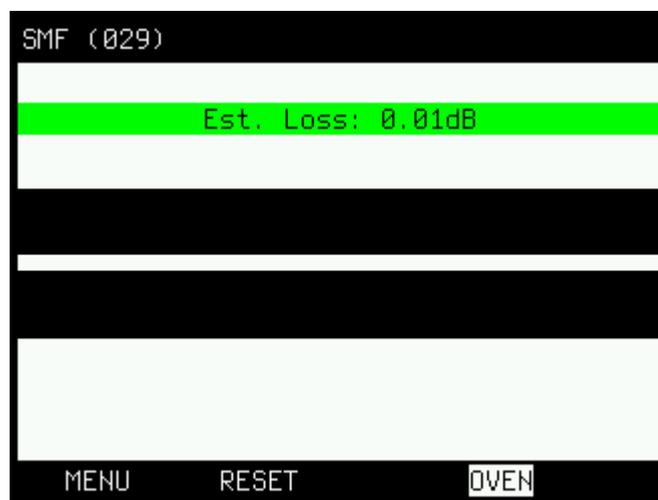
If estimated loss is larger than 0.1dB the splice is bad and has to be re-spliced.
