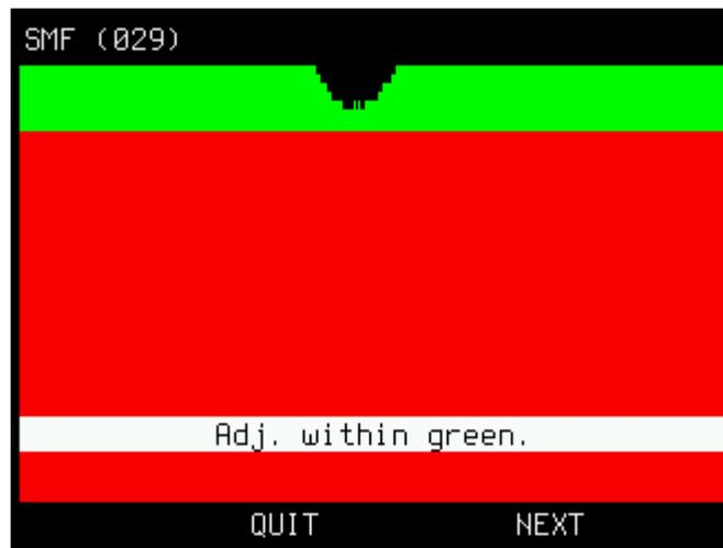
Adjust the upper electrode so that it is within the green area or just outside. But it must not be visible in the red area.
