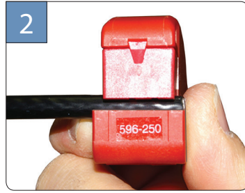
Using a fixed blade, prep tool in good condition, prepare cable to 1/4" x 1/4" dimensions. Use edge of tool if no stop
