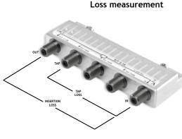
A signal is applied to the IN connector. For Tap Loss the output is measured on the other TAP connectors. For Insertion Loss the output is measured on the OUT connector.
