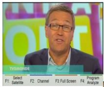
RADIO, and press F3 button to switch channel type (FTA/CAS/HD), and press F4 button to enter Channel Manger menu. In this menu, you can press F1 button to delete channels, press F2 button to move channels, and press F4 button or press EIXT button to exit channel manage menu.
