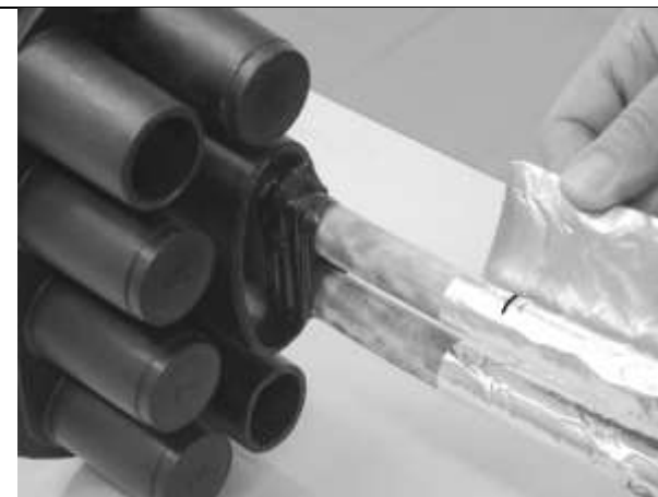
Match the mark of the aluminium protection foil with the mark on the cable. Wrap aluminium cable protection foil around the cable.
