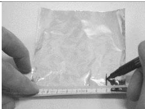
Mark the aluminium protection foil at 20 mm starting from the border.
