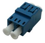
Our range of LC adapters have high precision alignment sleeves for improved reliability and better reconnectability. The LC adapters come with ceramic sleeves for both single mode and multimode. The housing is available in different colors with options for flange or flangeless body and metal or inbuilt clips.
