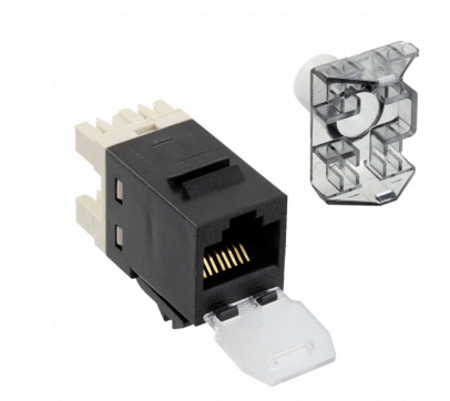
SL110 Series Modular Jack, RJ45, 8-position, category 6, T568A /T568B, unshielded, with dust cover, black
