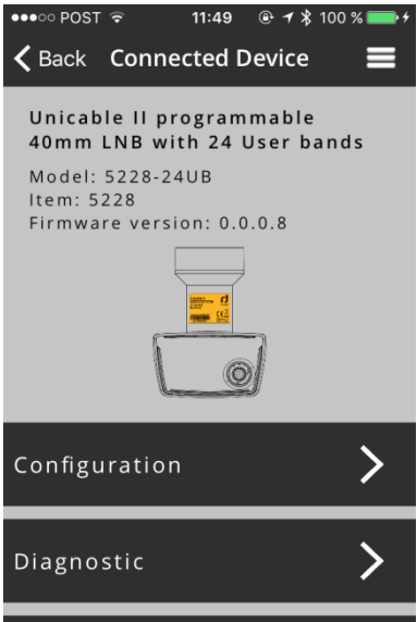
Figure 41: Unicable II™ Connected Device, LNB
